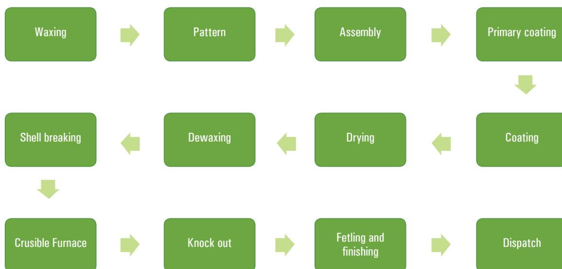
Various technologies such as wax injection press, jar mill, slurry coating drum, chiller, sand raining engine, dust collector blower, shell baking furnace, induction furnace, knockout machine, sand blasting machine etc. are used in the production process of investment casting.
